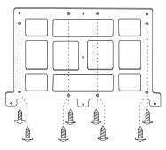
3. Match the position of installation bracket and installation plate with screw A.
