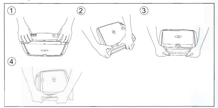
Begin by hooking the area and slide the cover over the pod. The cover will snap in place.
