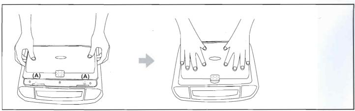
Open the screen and hook the two tabs (A) on the bottom edge of the screen. Snap the opposite side over the hinge.
