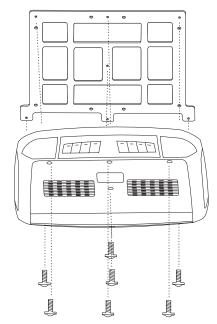
4. Tighten the unit with the supplied screw B.
